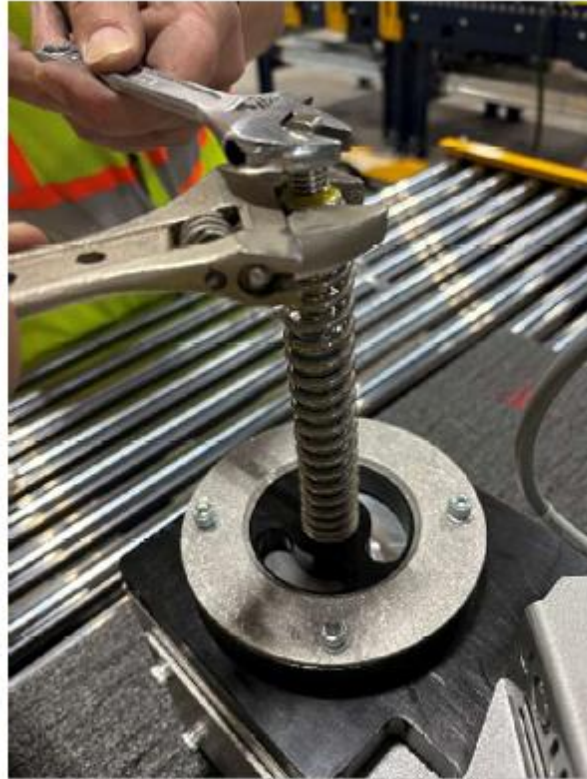
FIG 2: Pressure Adjustment Spring
