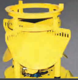
The remote crosshead power unit is mounted on the machine frame at conveyor level and is easily accessible from the work platform for service and routine maintenance. The power unit shroud dampens noise and protects components.
