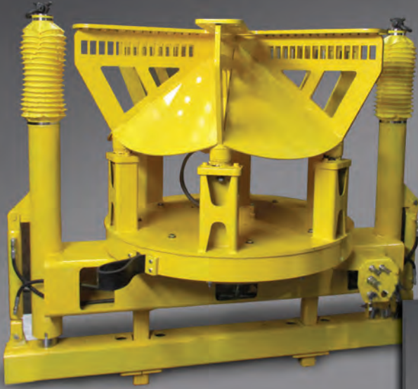
The hydraulic bell packer assembly features quick-change turning and vibrating standards for even more quality and efficiency in the pipe plant. Protective bellows on the shafts keep the guide system free from material contamination.
