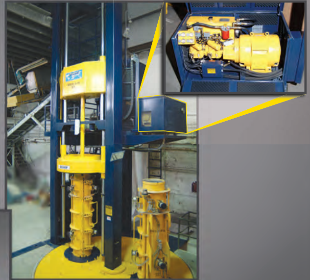
The remote crosshead power unit is mounted on the machine frame at conveyor level and is easily accessible from the work platform for service and routine maintenance. The power unit shroud dampens noise and protects components.
